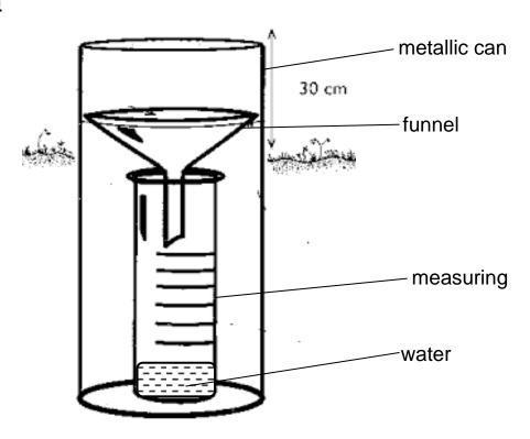
A rain gauge should be placed at least 15cm below the ground.
