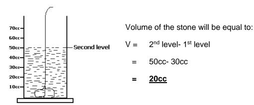
The volume of the stone is 20cc because when an object is lowered in water, it displaces an amount of water equal to its volume.
