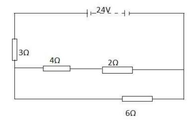
An accumulator of e.m.f. 24V and internal resistance of  $2\Omega$ , is connected to  $3\Omega$ ,  $4\Omega$ ,  $2\Omega$ , and  $6\Omega$  resistors as shown in the diagram above.
