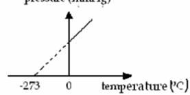
When the graph above is re-drawn with temperature converted to absolute scale, the graph now passes through the origin.
