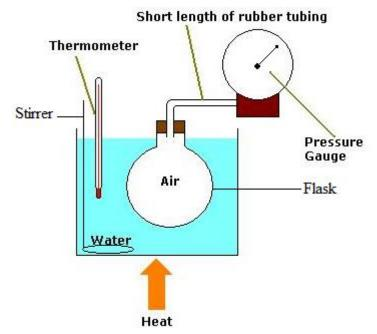
Dry air is trapped in a flask F and is connected to a pressure gauge.
