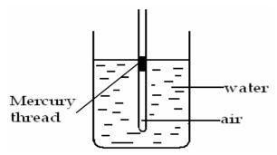
A graduated glass-tube containing air trapped below a mercury thread is immersed in a beaker of water and the water is heated as shown in the figure above.
