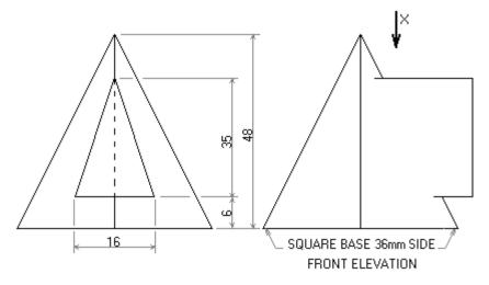
10 . The front and plan of a bracket are shown in the figure below. Draw an auxiliary elevation in the direction of arrow X. Sow hidden details.
