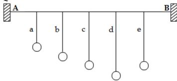
The diagram shows a stretched wire AB to which pendulums of lengths a, b, c, d, and e are attached
