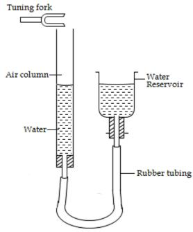
The length of the air column in the tube is altered by raising or lowering the reservoir. When the tuning fork vibrates it forces the air in the tube to vibrate at its own natural frequency forming resonance. The effect of resonance is a loud sharp sound.
