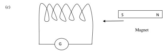
The diagram above shows a coil connected to a centre-zero galvanometer, G.
