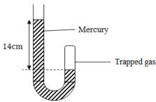
A gas is trapped by mercury in a J-tube at atmospheric pressure of 760mmHg as shown in the diagram above. Calculate the pressure exerted by the trapped gas in Nm<sup>-2</sup>. (2marks)
